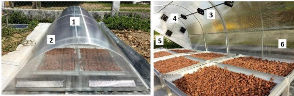
Figure 9: Study of a pilot project for cocoa bean drying using polycarbonate tunnels in Tabasco, Mexico (1. Polycarbonate cover with UV protection; 2. Windows allowing air in; 3. Fans to homogenize the internal heat; 4. Exhaust fans; 5. Tray holder; and 6. Trays) (Cerino & García, 2018)
