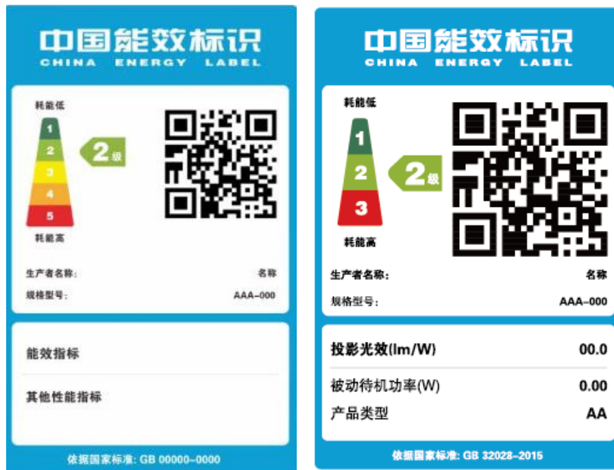
Figure 9: China - Energy Label with 5 levels (left) and Energy Label with 3 levels (right)
