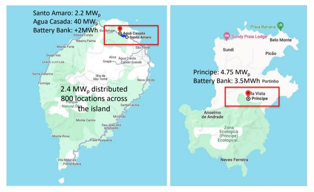
Figure 126: Tentative locations for central solar power plants with BESS in São Tomé and Príncipe
