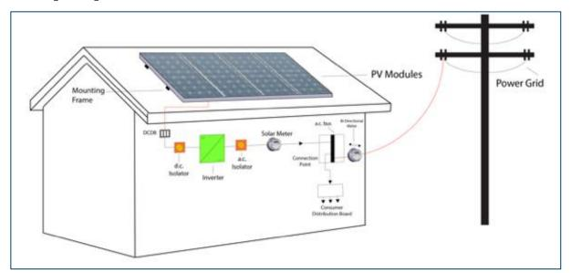
Figure 129: Net metering arrangement
