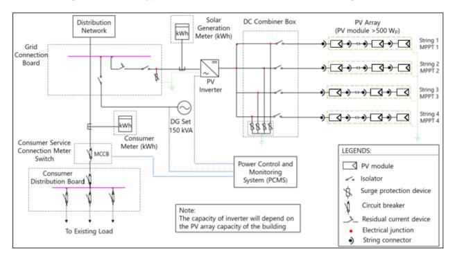
Figure 60: Single line diagram of rooftop PV system for Escola Secundaria Maria Manuela Margarido
