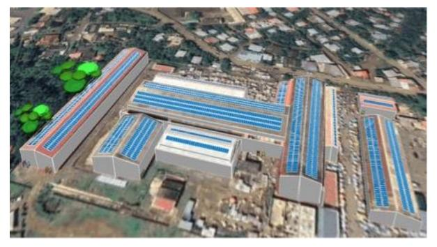
Figure 127: Site No. 15 (Mercado de Bobo Foro) with an estimated PV capacity of 937 kWp
