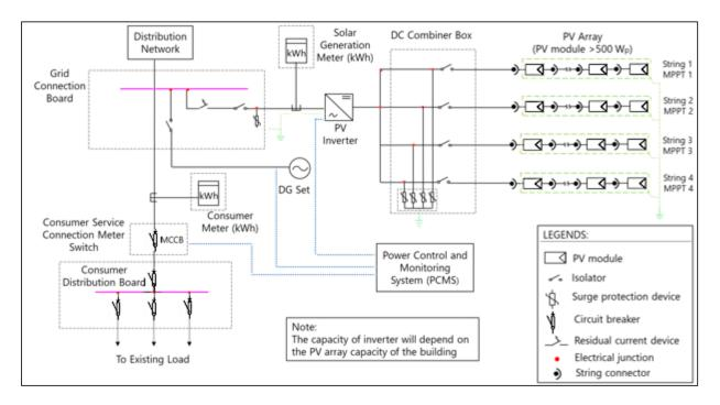
Figure 101: Single line diagram of rooftop PV system for Casa Da Cultura
