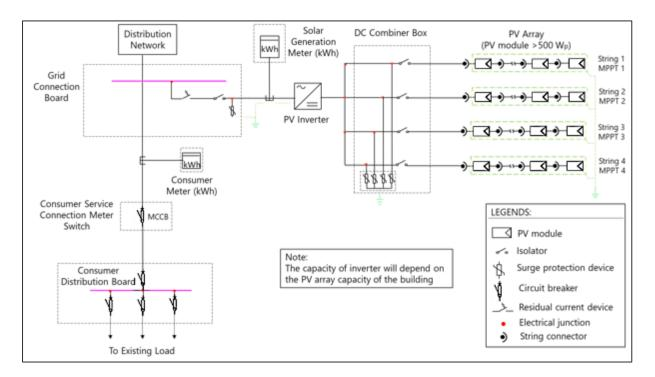
Figure 95: Single line diagram of rooftop PV system for Escola De Padrão
