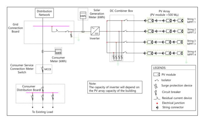
Figure 75: Single line diagram of rooftop PV system for Escola Secundária De Neves
