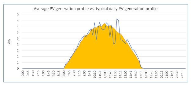
Figure 111: Solar power generation profile – average and actual on a typical day
