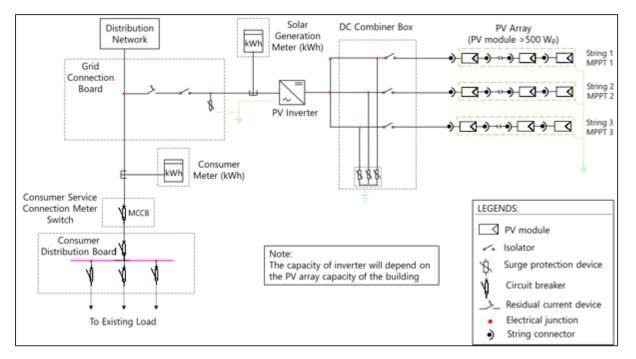
Figure 86: Single line diagram of rooftop PV system for Camara Distrital De Lembá
