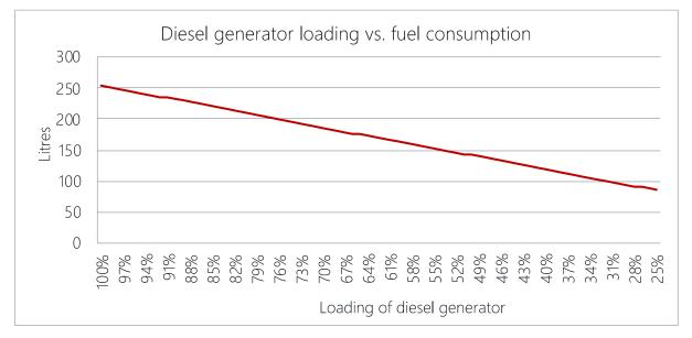
Figure 109: Diesel generator fuel consumption vs loading (1 MW plant) (Source: Caterpillar)
