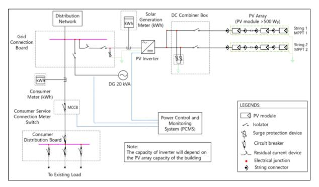
Figure 21: Single line diagram of rooftop PV system for Procurador/Ministério Publico
