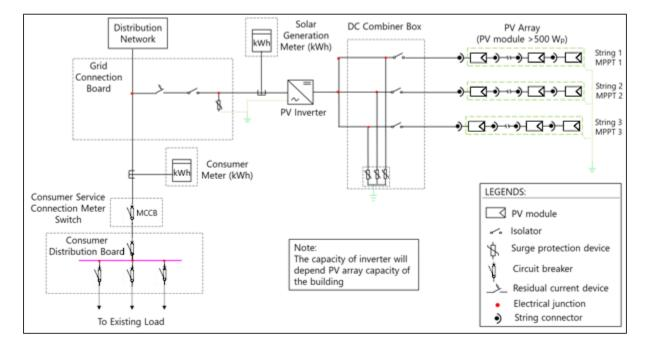
Figure 51: Single line diagram of rooftop PV system for Escola Secundaria De São João Dos Angolares
