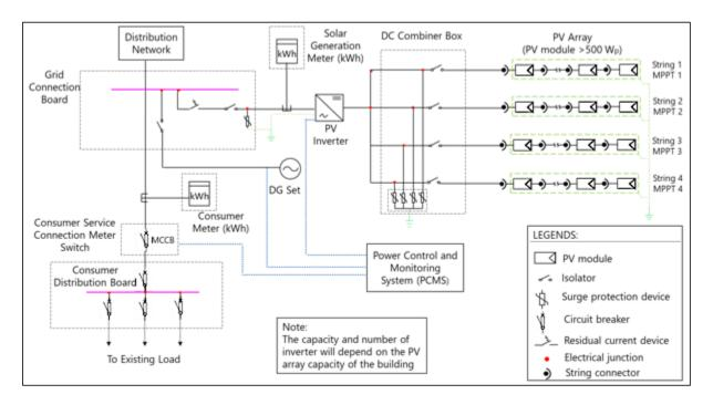
Figure 30: Single line diagram of rooftop PV system for Hospital Dr. Aires De Menezes
