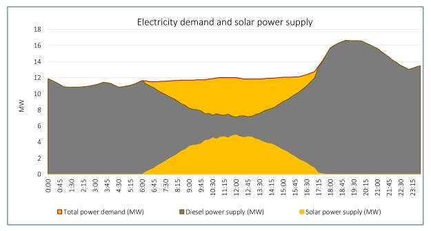
Figure 110: Typical day load profile and average solar power contribution
