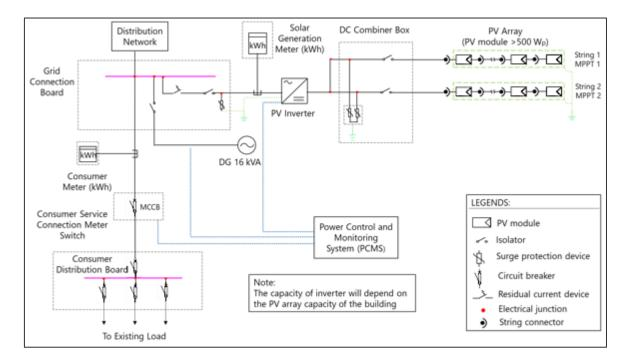
Figure 27: Single line diagram of rooftop PV system for Autoridade Geral De Regulaca (AGER)
