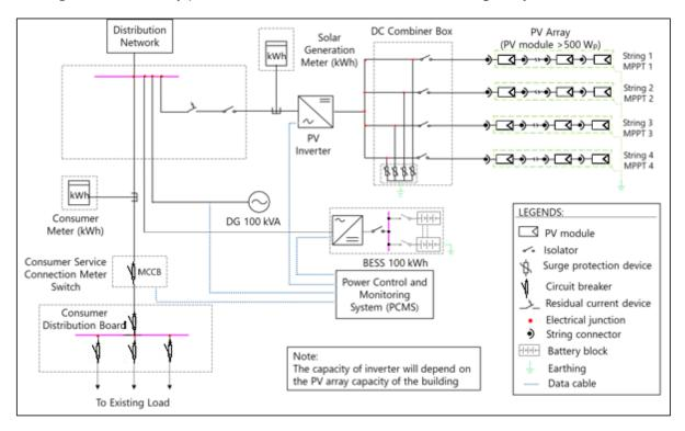
Figure 42: Single line diagram of rooftop PV system for Tribunal De Contas
