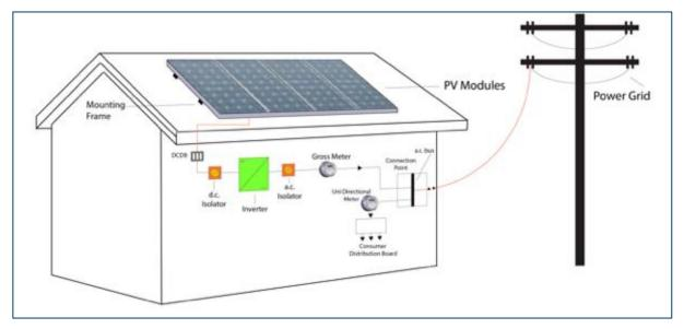
Figure 128: Gross metering arrangement
