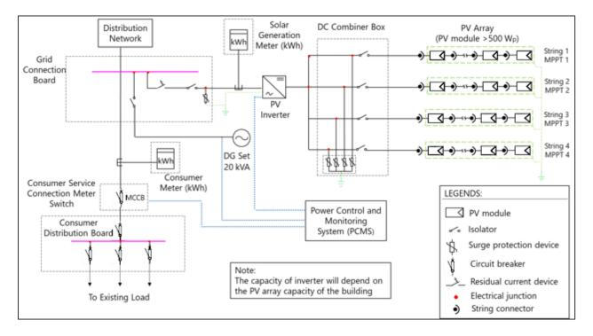
Figure 54: Single line diagram of rooftop PV system Posto De Saúde
