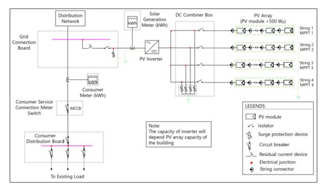
Figure 45: Single line diagram of rooftop PV system for Liceu Nacional De Santana
