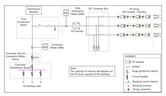
Figure 81: Single line diagram of rooftop PV system for Posto De Saude De Lembá
