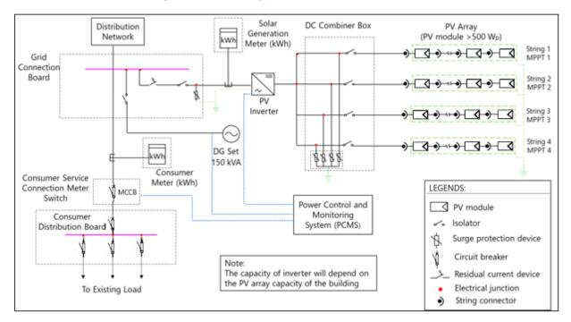
Figure 66: Single line diagram of rooftop PV system for Liceu Mé Chinhô
