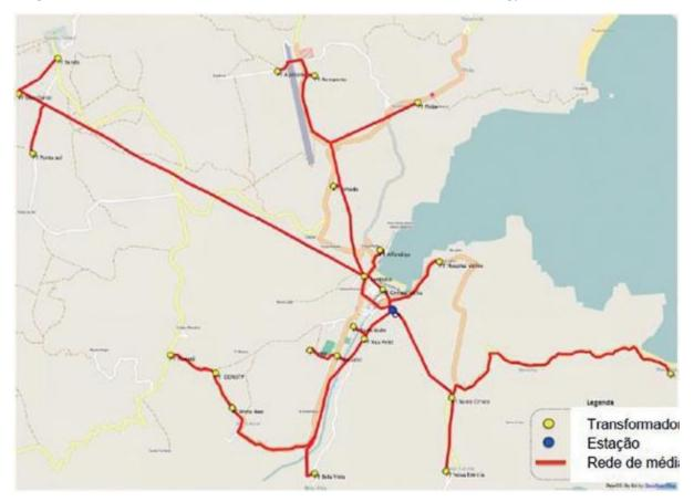
Figure 9: Electrical distribution network of Príncipe (Source: Ricardo Energy & Environment, 2018)
