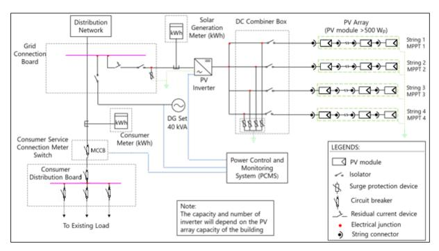
Figure 36: Single line diagram of rooftop PV system for Liceu Nacional
