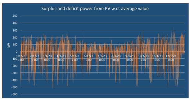
Figure 113: Surplus and deficit power from 1 MW<sub>p</sub> PV power plant w.r.t average value
