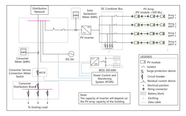
Figure 98: Single line diagram of rooftop PV system for Banco Internacional De São Tomé & Príncipe
